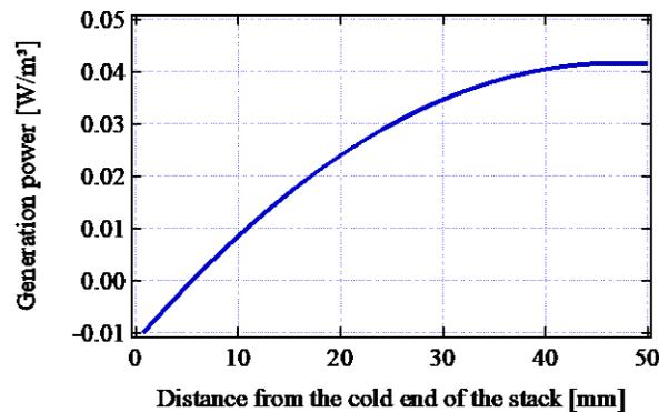
**Figure 5.** Generated power distribution immediately after starting oscillation
